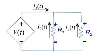
Our special case, signals of the form: V(t) or  $I(t) = Ae^{st}$ where s can be a real or complex number
