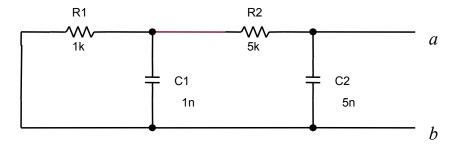
Find and plot the impedance  $Z_{ab}(j\omega)$  as function of  $\omega$ . Use Matlab to calculate the Bode plot.
