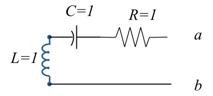
Find and plot the impedance  $Z_{ab}(j\omega)$  as a function of frequency. Use Matlab to calculate the Bode plot.
