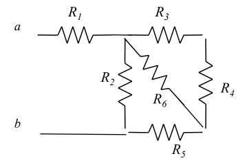
Find the total resistance  $R_{ab}$  for this infinite resistive network
